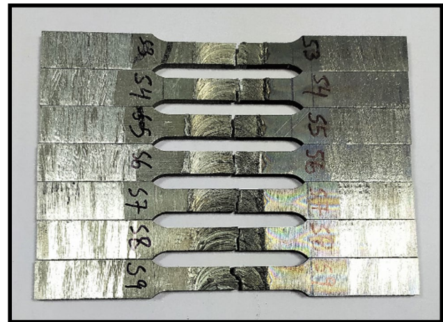
Fig. 18 Crack position of failure of tensile specimen S3 to S9 (between HAZ and SZ)
