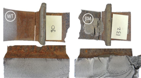
Fig. 18 Failure locations (WT: Weld Toe, BM: Base Material) and Fatigue strength ( P_s = 50\% ) of TS in the AW and HFMI treated state [4, 5]
