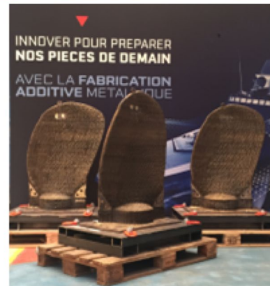
Fig. 8 Production of the series blade preforms
