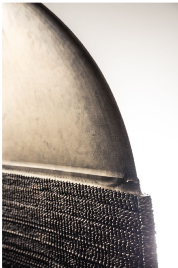
Fig. 2 Comparative view of the rough deposit state and the machined state
