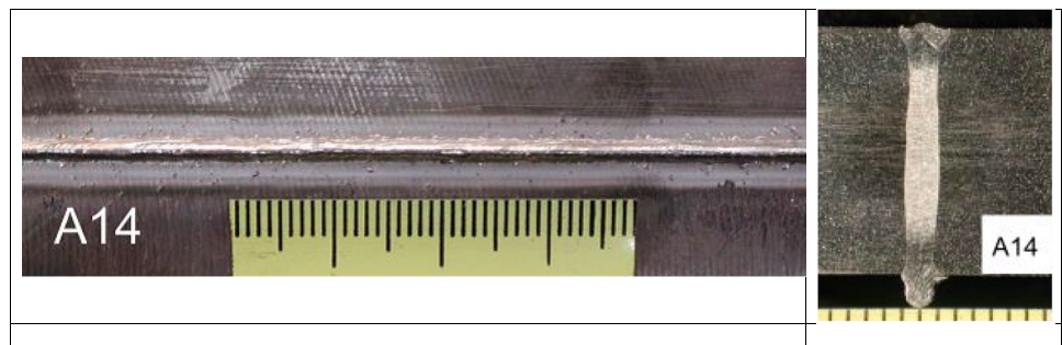
Fig. 11 Bead-on-plate weld of a 14-mm-thick test piece A14: a) root side of the weld and b) macro cross-section. Beam current used: 52.3 mA. In the scale strip, one interval corresponds to 1 mm
