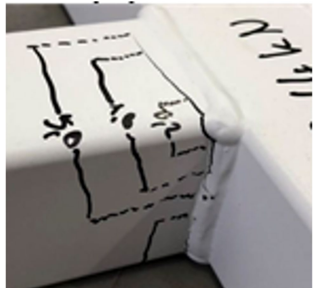
Fig. 4 Typical failure pattern and crack lengths at different displacement increases, values in mm
