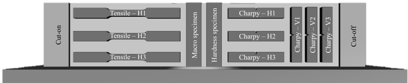
Fig. 3 The locations of the test specimens on the 16 mm thick WAAM-Wall steel material. The length of the wall was 320 mm while height of the wall was approx. 60 mm with the thickness of 16 mm
