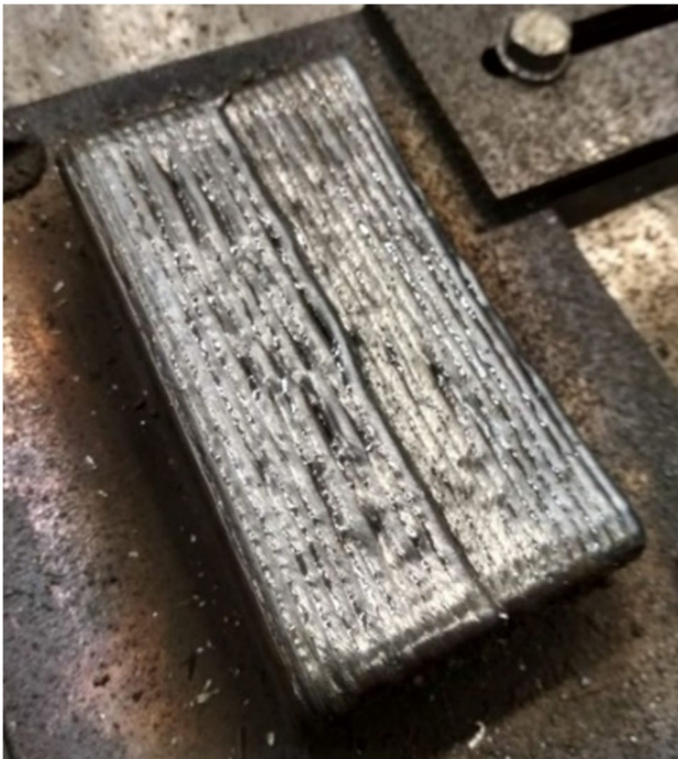
Fig. 5 Block (HI 0.186 kJ/mm) during deposition
