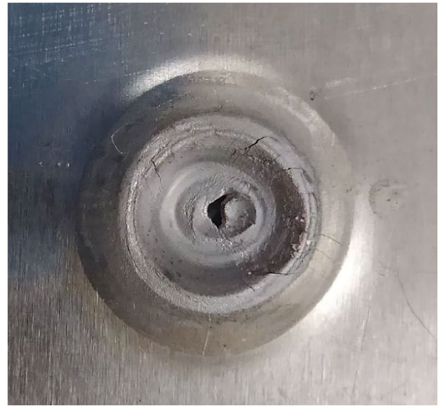
Fig. 4 Failure behaviour of the joints with maximum shear strength for (a) Al-Cu and (b) Cu-Al configurations
