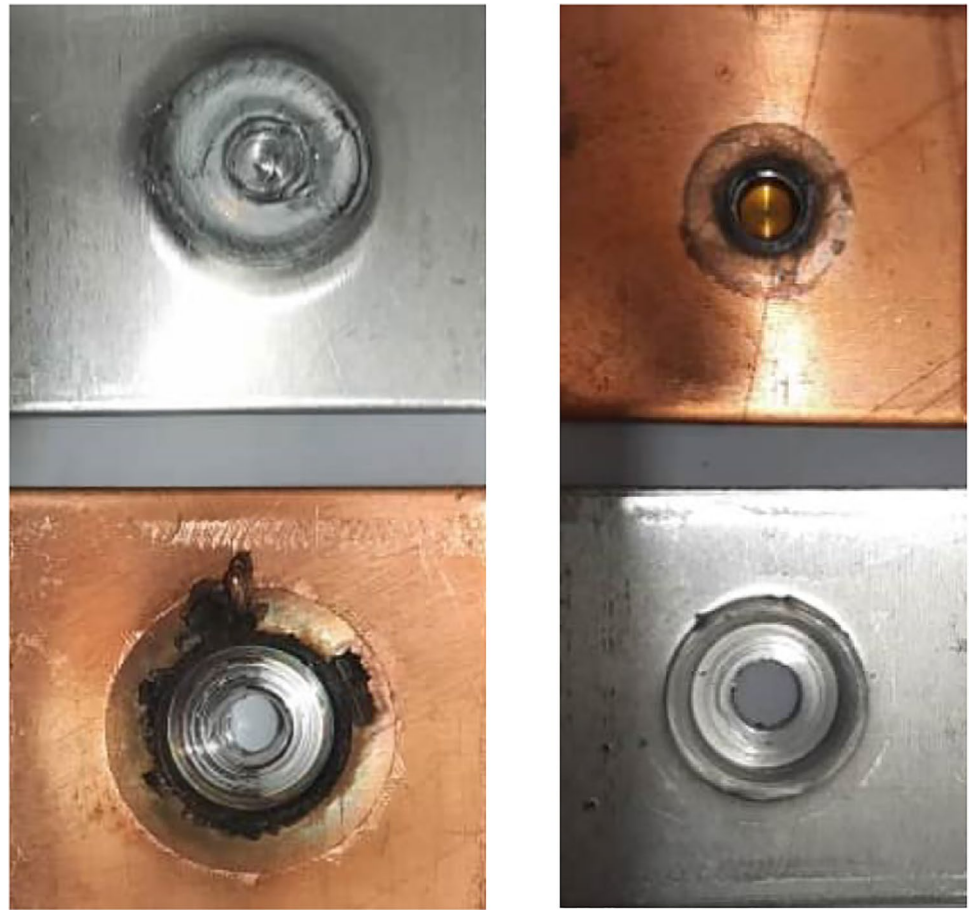
Fig. 16 Photographs of the failed (a) Cu-Al and (b) Al-Cu specimens, welded at optimum condition
