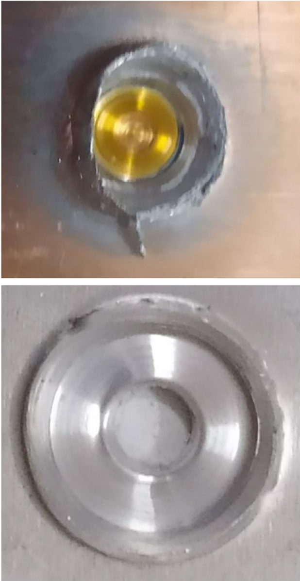
Fig. 6 View of the fractured surfaces for Al-Cu configuration with maximum shear strength
