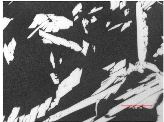
Fig. 8 Microstructure in HAZ etched with Lichtenegger & Blöch LB1, temperature > 60 °C (140 °F) (ferrite in dark and austenite in white)
