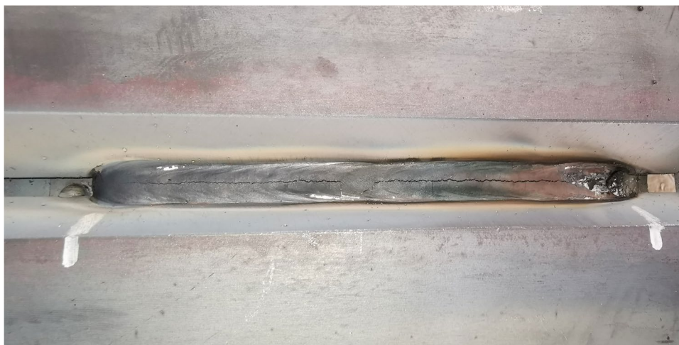
Fig. 11 Solidification crack detected with a duplex flux-cored wire in a modified version of the FISCO test, where rapid welding can be performed against ceramic backing [114]
