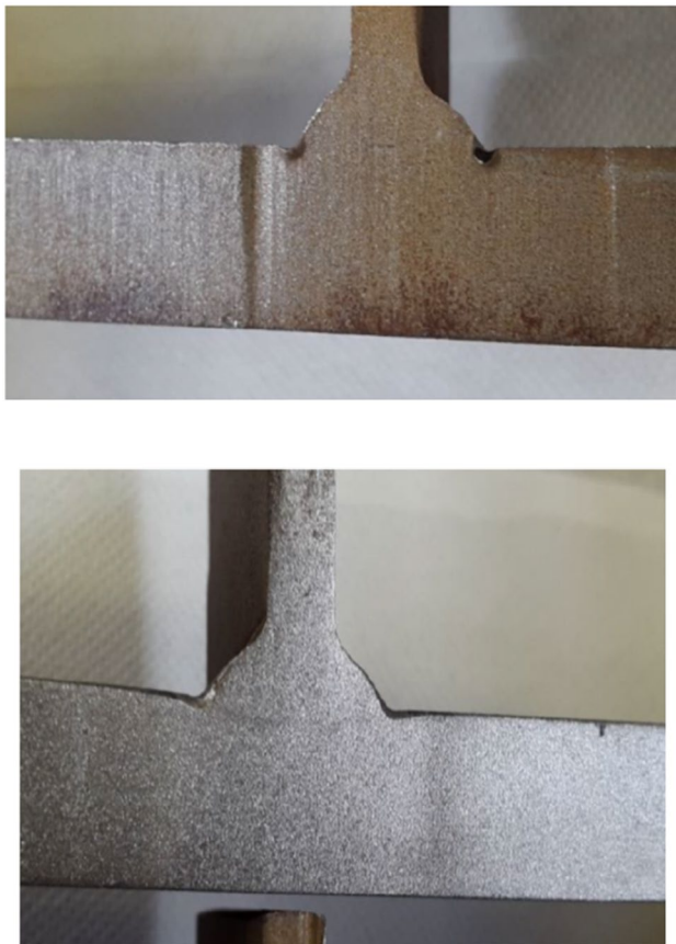
Fig. 4 Test specimen, HFMI-treatment with and without finishing of the edges
