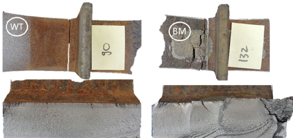
Fig. 10 Failure locations of the AW series (WT) and the HFMI series (BM) as well as typical fracture pattern of the one-sided TS
