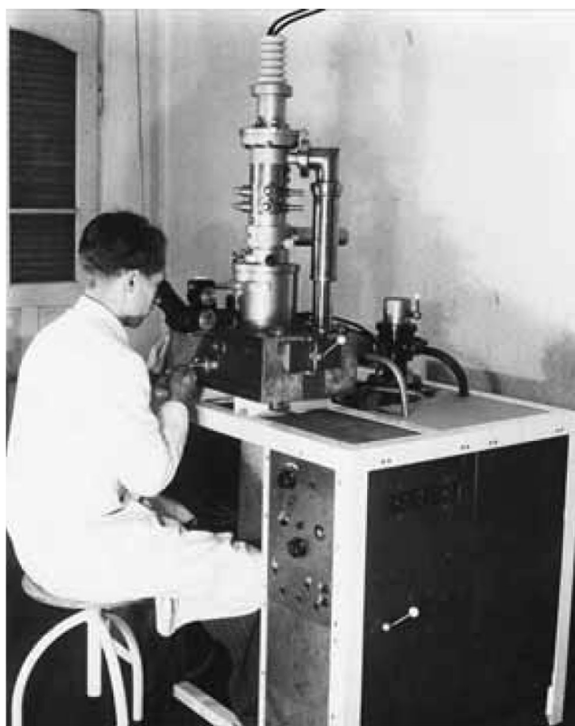
Fig. 4 Lab prototype of an electron beam welding machine, 1951 [1]
