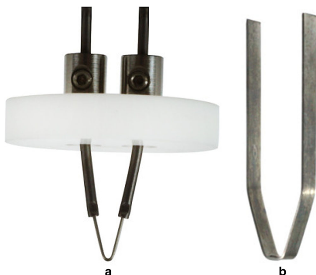
Fig. 40 Hairpin filament (a) and ribbon filament (b) [237]
