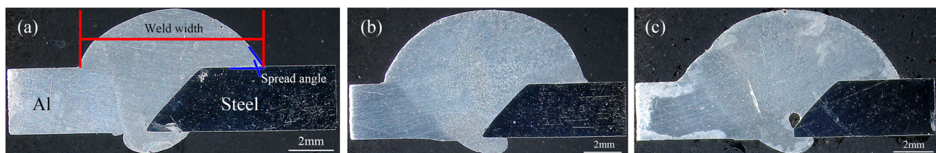
Fig. 5 Macrographs of the seam with the different wire feed rate (welding speed: 400 mm/min): a 5/min, b 7 m/min, c 7.5 m/min
