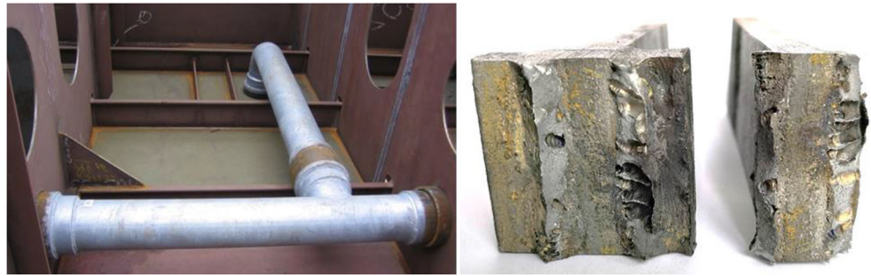
Fig. 1 Example of galvanized structures in shipbuilding: ballast water pipes (left). Problems by welding galvanized structures: fracture surface of a welded hot-dip galvanized cruciform joint ( t = 10 mm) with numerous pores in weld metal (right)
