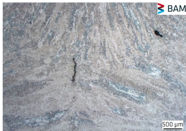
Fig. 10 Weld defects found with metallographic analysis of the 40-mm modTTS with high HD
