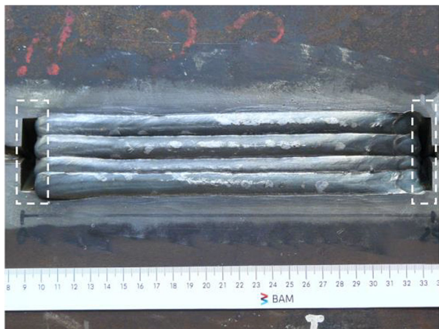
Fig. 9 Welded 40-mm modTTS with gaps in the start and end of the weld seam
