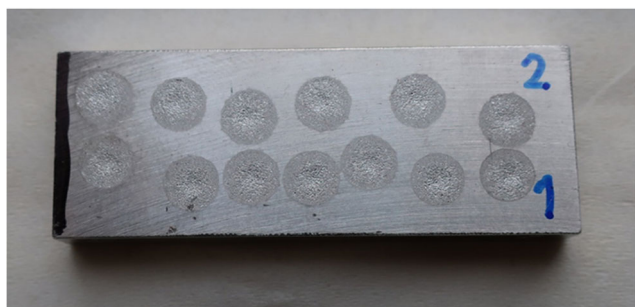
Fig. 5 Cross-section of the 10-layer, 5-bead block showing two lines of OES spots. Line 1 shows the locations close to the substrate, and line 2 shows the locations close to the top
