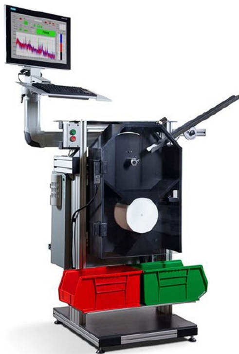
Fig. 8 RAM setup used to test the Co–Cr lattice structures
