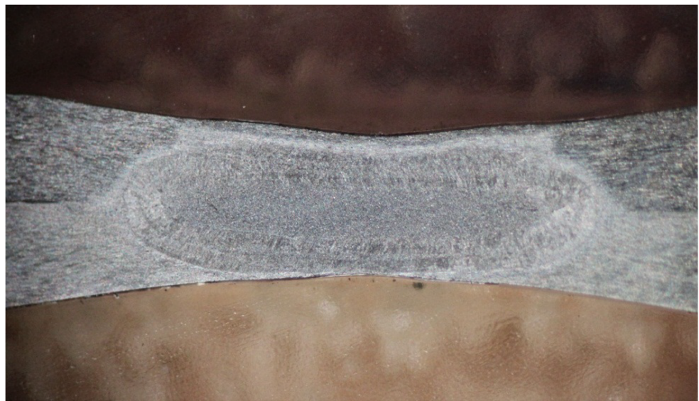
Fig. 10 Cross section of a welded joint of t = 1 mm AA 7075 alloy (magnification \times 16 )
