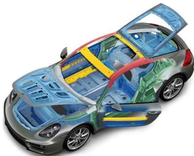
Fig. 1 Car body where the blue colours represent the high strength aluminium alloys [3]
