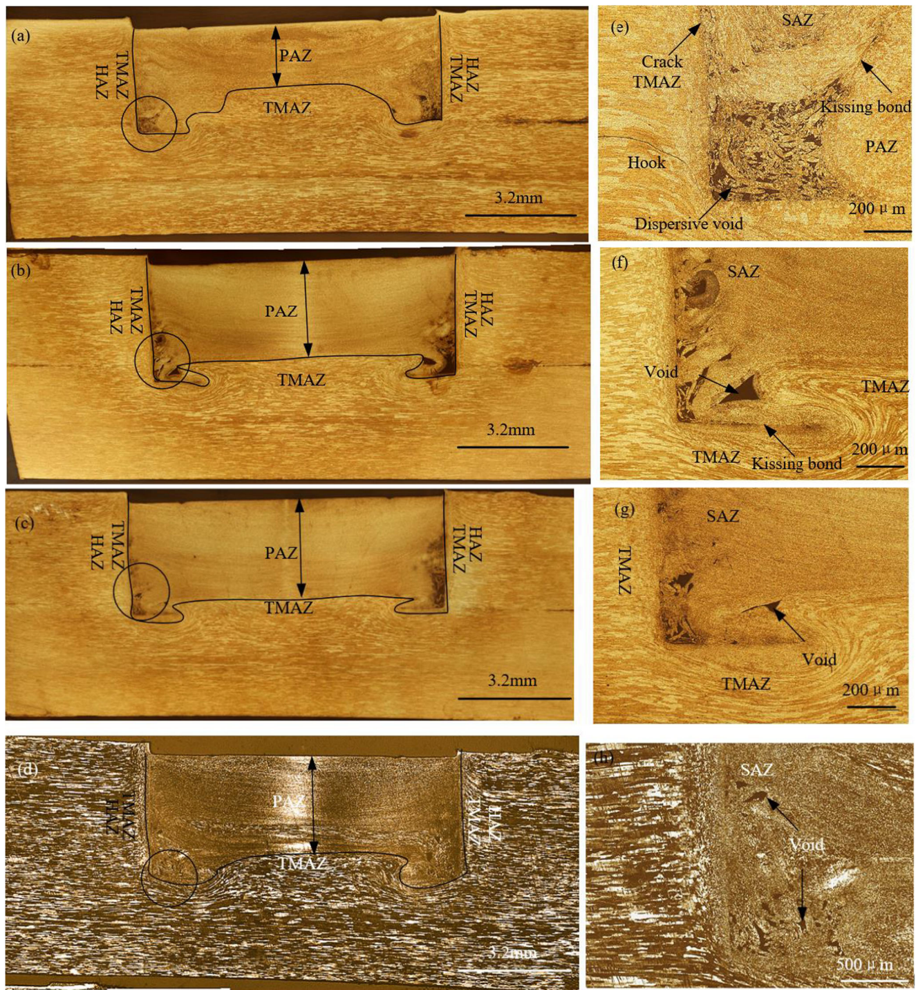
Fig. 4 Cross-sectional structures of refill FSSW joints at different plunge depths: a, e 3.4 mm; b, f 3.6 mm; c, g 3.8 mm; d, h 4 mm
