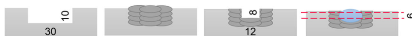
Fig. 2 Manufacturing route: Building up an all-weld metal zone. A disc with 6 mm thickness (red dashed line) subject to arc heat treated and the final bead is metallurgically investigated (bright blue)
