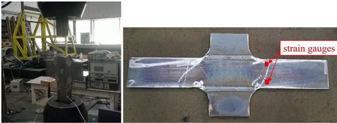
**Fig. 8** A broken specimen in the pulsator and the strain gauges on the II-type specimens
