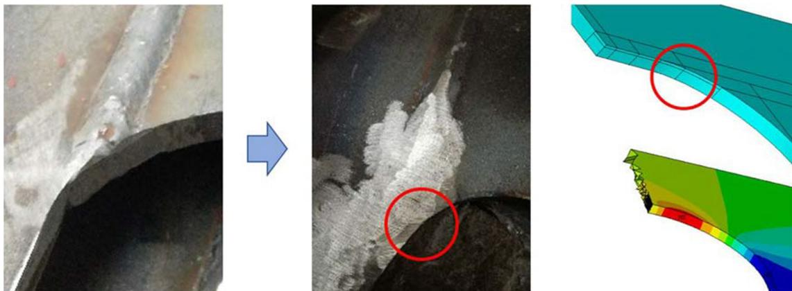
Fig. 16 Geometry modification by disc grinding and the numerical model
