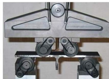
**Fig. 3** Geometry and test layout of the T-joint specimens [18]
