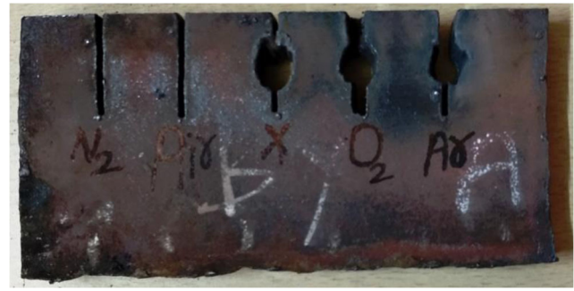
Fig. 11 Kerf geometries on the workpiece
