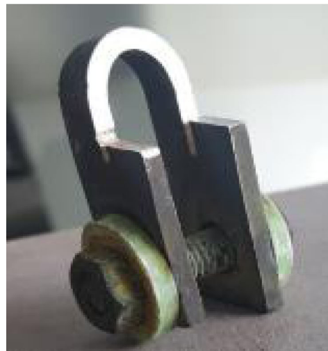
(b) - Perspective view of B Electrode weld CSCC sample 2 sectioning
