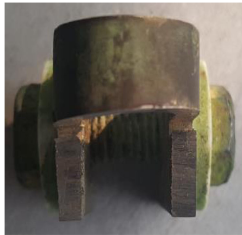
(a) – B Electrode weld CSCC sample 2 sectioning
