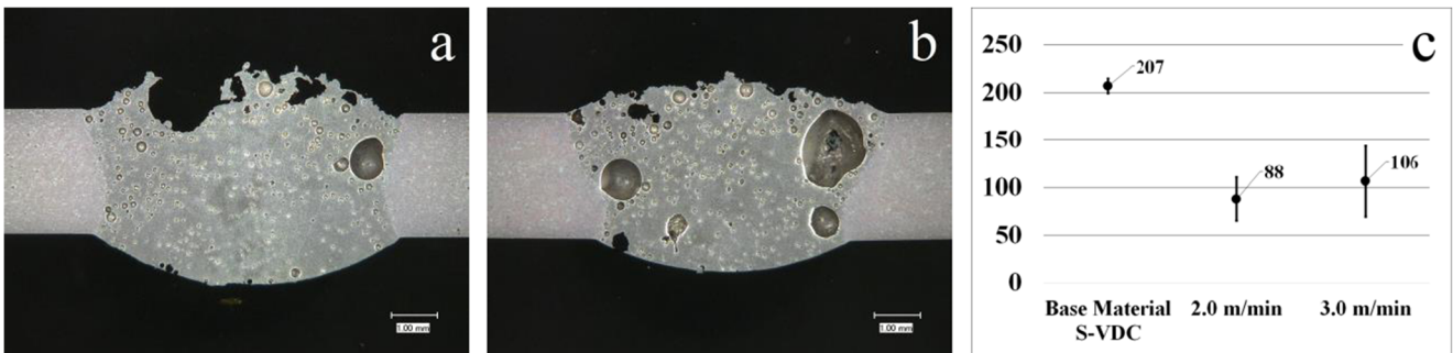
Fig. 6 Macrograph of NV-EB welded Silafont-36 vacuum die cast S-VDC samples with a 3.0 m/min, b 2.0 m/min welding speed, and c mean tensile strength with standard deviation
