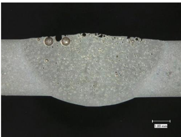
Fig. 4 Macrograph of NV-EB welded Silafont-36 vacuum die cast S-VDC sample with 1.6 m/min
