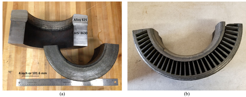
Fig. 1 a 8630/625 dissimilar metal weld coupon. b Coupon after EDM machining of DHCT samples
