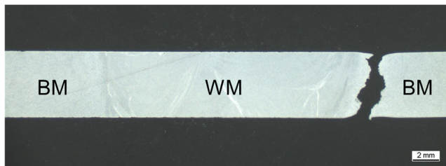
Fig. 4 Macro-picture of the fractured creep sample
