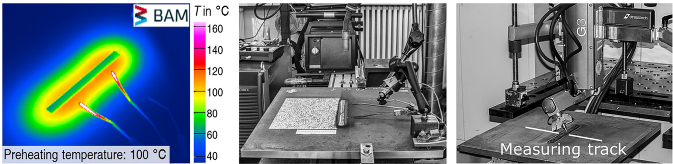
Fig. 4 In situ analyses of the temperatures and stress-strain fields adjacent to the weld, while preheating, welding and cooling, local residual stress analyses via XRD [5]
