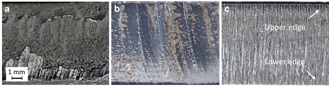
Fig. 5 Cut surfaces of steel S355M (8 mm thick): a oxygen cutting, b plasma cutting, and c laser cutting
