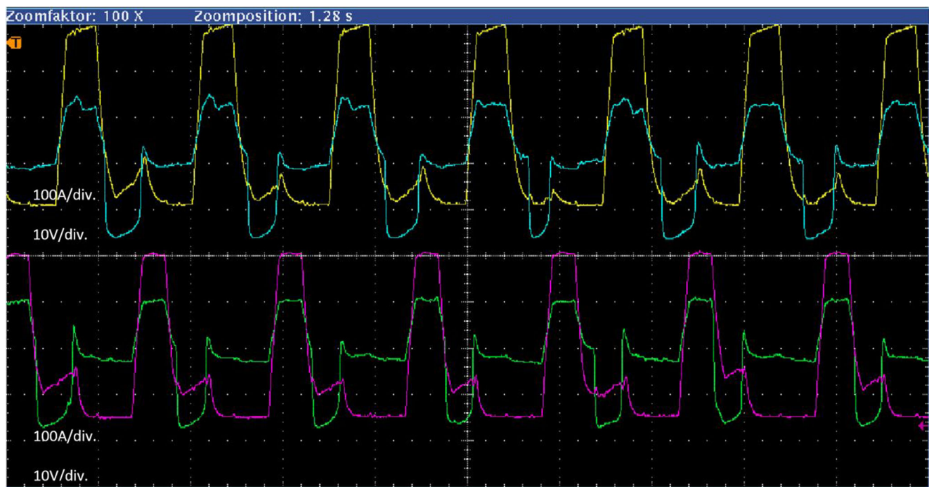
Fig. 13 Welding voltage (lower values) and current (higher values) for both wire electrodes through applying advanced LTHW and using different wire electrode diameters at same wire feed rate. Upper portion shows leading arc; lower portion depicts trailing arc
