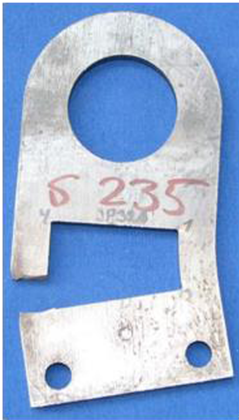
Fig. 15 Typical failure of the test specimen
