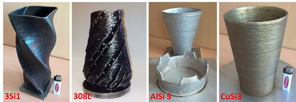
Fig. 2 CMT–MAM examples for thin-walled simple 3D–shapes out of different filler wires (unalloyed steel, stainless steel, aluminum, copper alloy)
