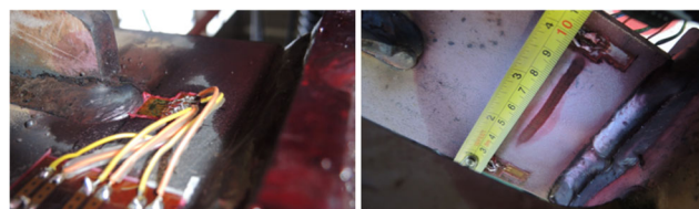
Fig. 24 Exemplary picture of applied stress gauges. At weld toe of the longitudinal stiffener (left), stress gauges for machine control on the opposite bottom side with crack highlighted through penetration testing (right)
