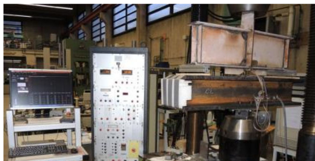
Fig. 23 Experimental setup for fatigue testing of 1:2-scaled components
