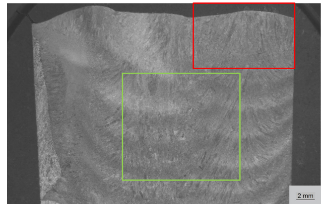
Fig. 9 Microstructure and position of hardness measurements
