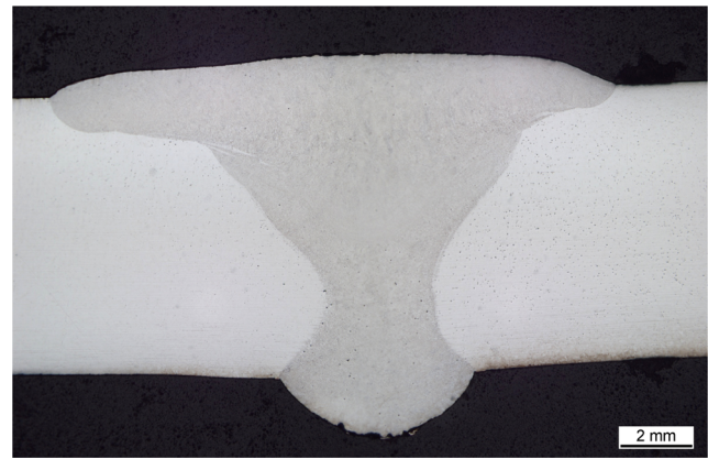
Fig. 5 Micrograph taken from a tubular butt-weld at \varphi = 135^\circ
