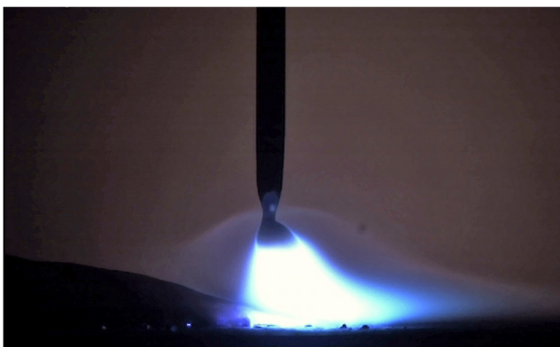
Fig. 2 Arc anchored at the end of the droplet when the wire is the anode
