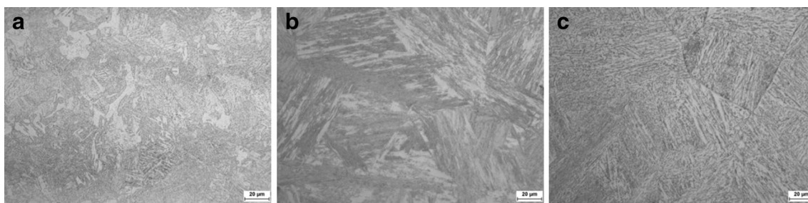
Fig. 2 a BM, (b) M HAZ, and (c) B HAZ
