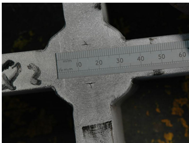
Fig. 2 Measurement of lack of penetration using MPI
