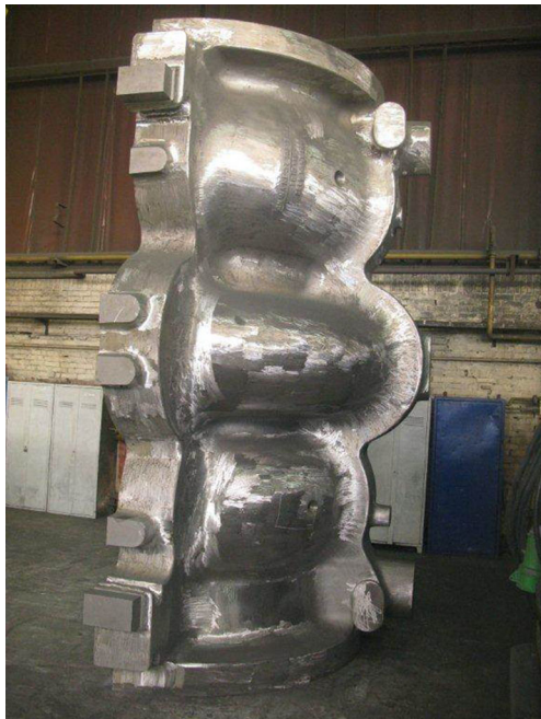
Fig. 1 CB2 IP inner casing manufactured at voestalpine foundry Linz [3]
