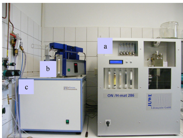
Fig. 3 CGHE hydrogen analyzer with a G8 Galileo instrument, b infra-red furnace, and c mass spectrometer
