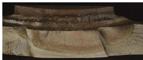
Fig. 17 Section through crack location 5 in specimen 3
