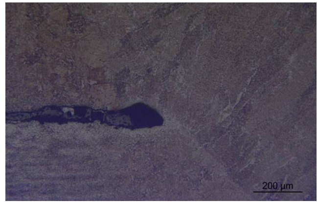
Fig. 26 Typical sample from weld root after testing. The weld is to the right of the opening
