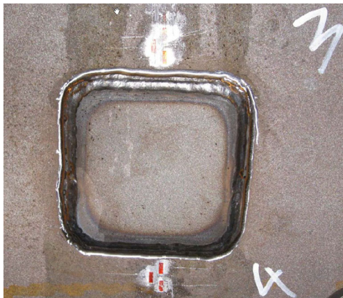
Fig. 6 Ground quadratic doubling plate
