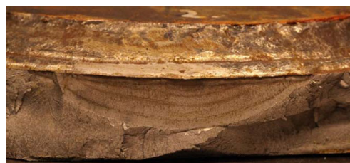
Fig. 19 Section through crack location 2 in specimen 5
