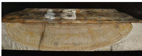
Fig. 18 Section through crack location 1 in specimen 5
