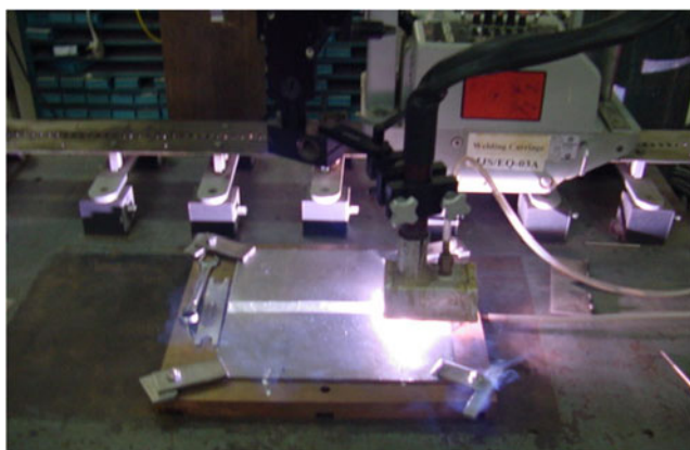
Fig. 2 ATIG welding of titanium in progress
