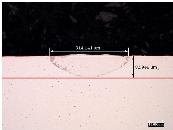
(a) Measurements of melt pool width and depth
