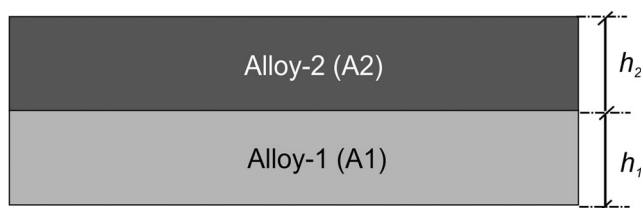
Fig. 2 Schematic of an FGM system involving two metallic alloys with equal thickness
