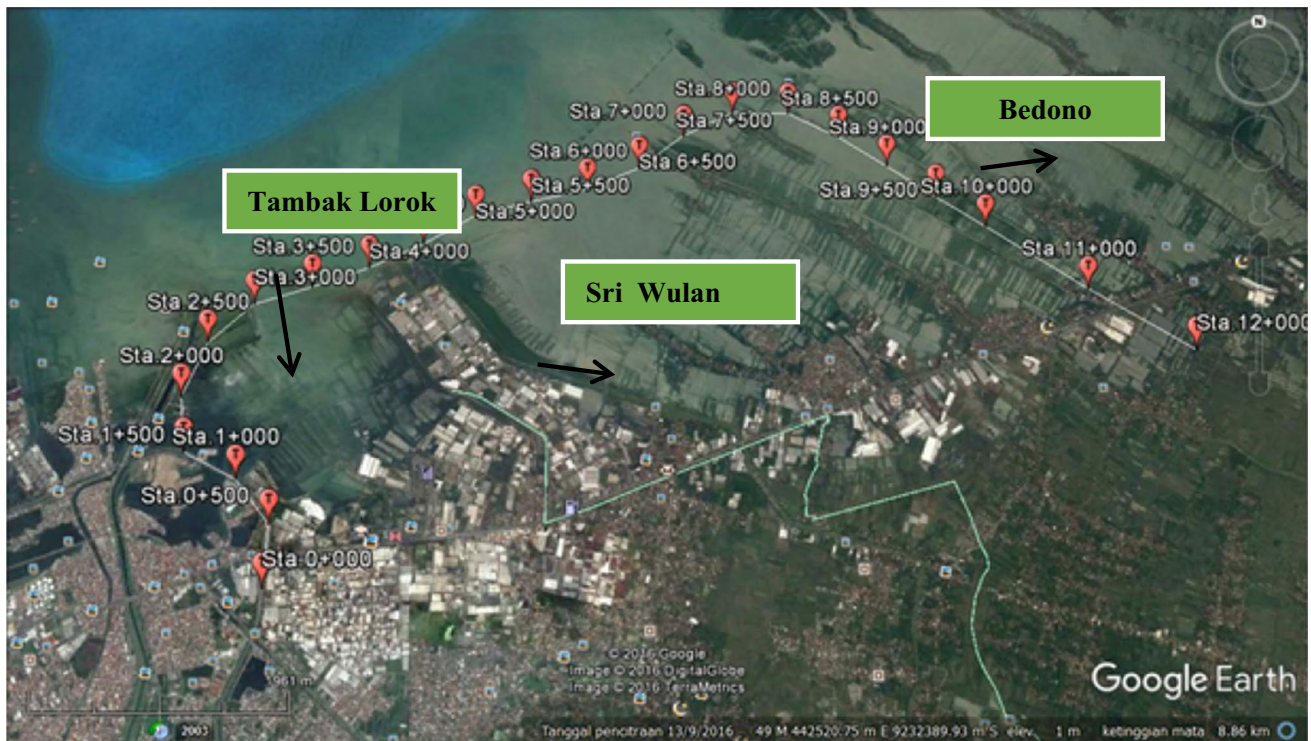
Fig. 3 Sea wall and toll road integration track. The figure shows the initial tract of sea wall and that the toll road integration with 8 km is a sea wall with a height of 5 m. It starts near Tambak Lorok Semarang
