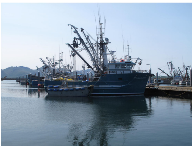
Fig. 4 Modified "super" 58' salmon seiner and cod/pollock trawler
