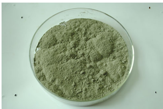
Fig. 8 Photo of the as-prepared SiC powders by carbothermal reduction at 1800 °C for 2 h.
