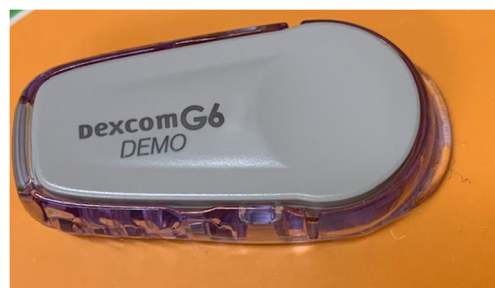
Fig. 2 Continuous glucose monitoring (CGM) Dexcom G6 (transmitter and sensor)
