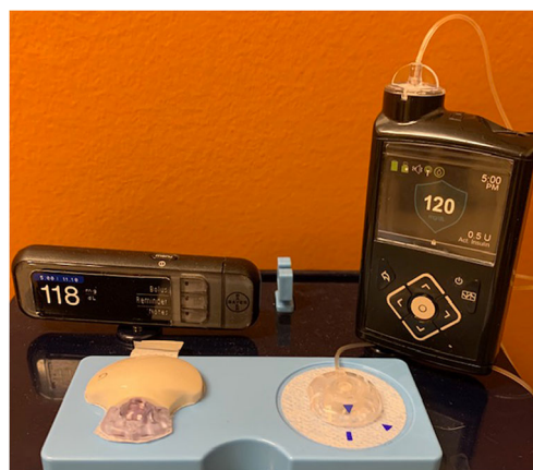
Fig. 1 Hybrid closed-loop system, Medtronic 670G (sensor, insulin pump, and glucometer)
