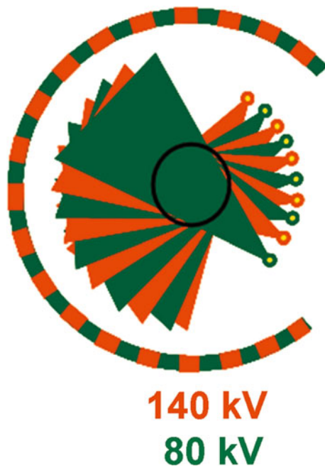
Fig. 11 Principle of fast kV-switching to acquire dual energy CT data
