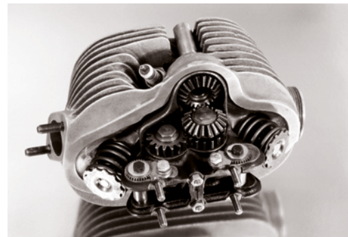
1953 Cylinder head with valve control in the BMW 253 RS
