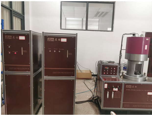
Fig. 2 ZTRE-210 microcomputer-controlled three-axis rock tester
